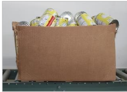
Image 2. The box is filled past the folding flaps, and is ripped, making it likely to break when lifted, and causing the cans to fall out.
