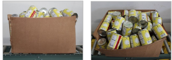
Image 2. The box is filled past the folding flaps, and is ripped, making it likely to break when lifted, and causing the cans to fall out.
